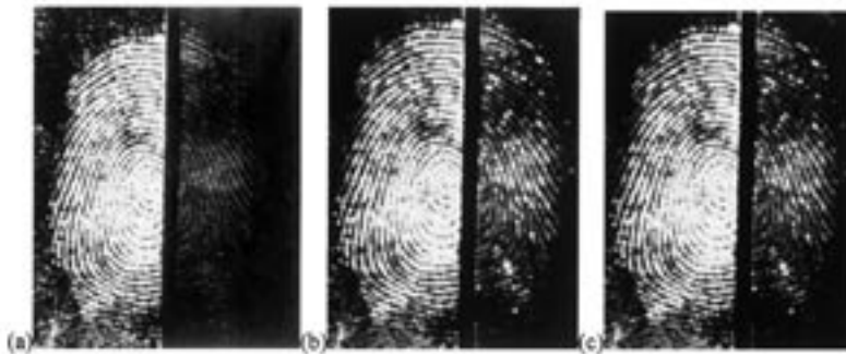
FIG. 4—Fingerprints developed using benzo[f]furoninhydrin/DFO at (a) 505/555 nm; (b) 530/590 nm, and (c) 555/610 nm at room temperature on manilla folders.
